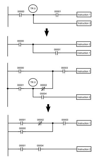
**Note** TR bits are only used when programming using mnemonic code. They are not necessary when inputting ladder diagrams directly. The above limitations on the number of branching points requiring TR bits, and considerations on methods to reduce the number of programming instructions, still hold.
